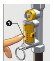
B. Use the ring (2) to open the obturator that shuts off the flow of medium in the flow meter (3) under normal operating conditions.
